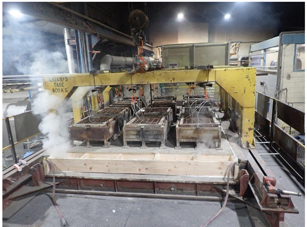
The unexposed face of the floor assembly after 68 minutes of testing
