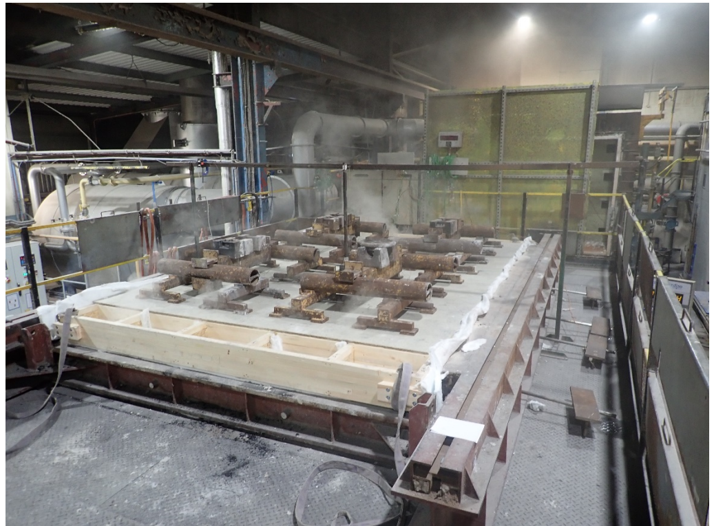
The unexposed face of the floor assembly after 36 minutes of testing
