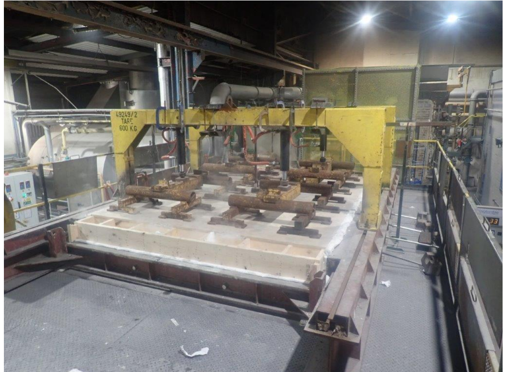
The unexposed face of the floor assembly after 26 minutes of testing
