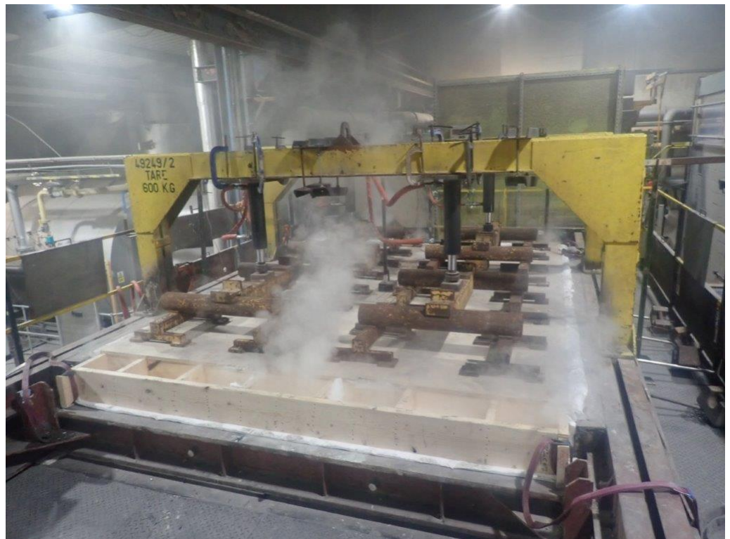
The unexposed face of the floor assembly after 100 minutes of testing
